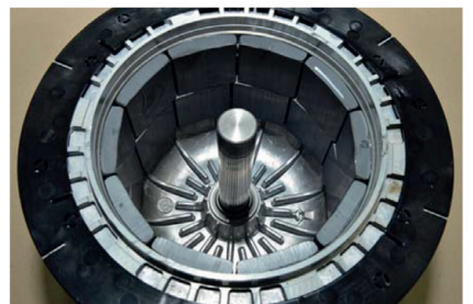
Rotor made of die-cast aluminum with plastic plate (not shown) on the ring.
