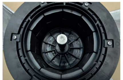
Steel rotor with plastic cooling wheel.
