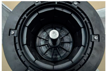
Steel rotor with plastic cooling wheel
