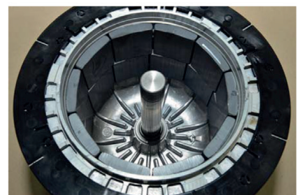
Rotor made of die-cast aluminum with plastic plate (not shown) on the ring.
